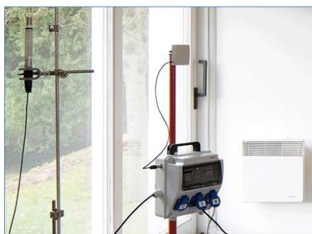
Figure 6: Test of a protocol to assess the energy performance of a completed building (Photo credit: CSTB)
