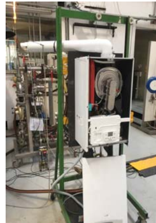
Test for the certification of a boiler In CETIAT laboratory
